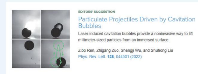
cavitation bubble of diameter about 5 mm by a pulsed laser in the neighborhood of the particle. Using high-speed photography, they observed that the particle was lifted from the immersed surface like a projectile with a controllable vertical displacement depending on the size and the position of the cavitation bubble.
